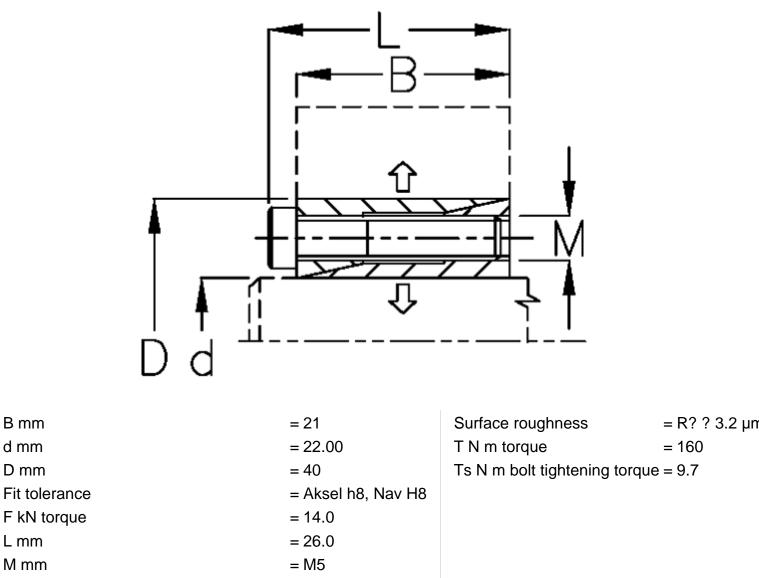
P N/mm2 surface pressure on shaft/hub = 70
